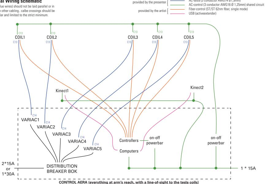
This diagram is meant to provide an overview of the different signals and feeds used by the installation. While the general layout of this diagram makes sense, it is not an accurate spatial reference. A proper schematic should be derived based on the plam of the venue.
